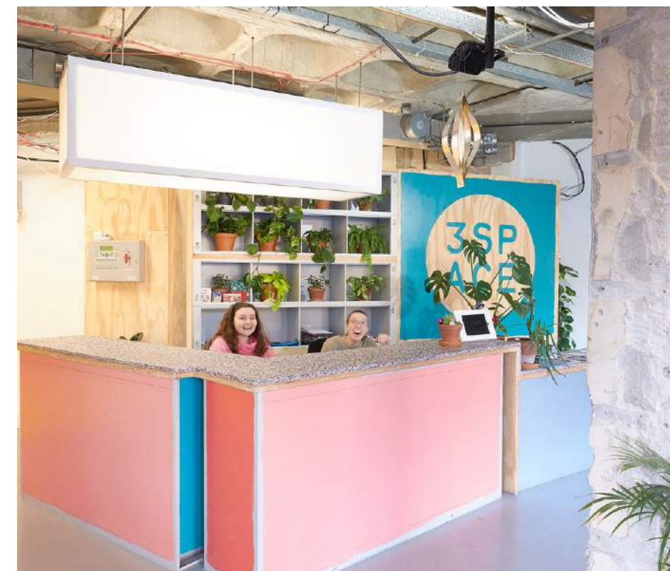
Filing cabinets that were already in the building were repurposed and converted into a reception desk topped with recycled plastic sheet material. A similar approach was taken wherever possible throughout the building
